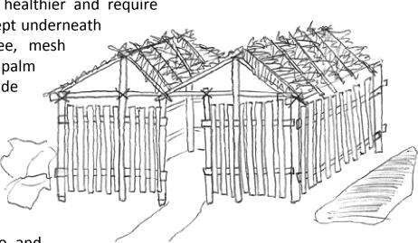
recycled building materials. Save on expenses by avoiding cement, metal, plastic and other inorganic materials. The PD greenhouse is built almost entirely out of bamboo and palm fronds which are ideal building materials because they are all natural, easy to work with, inexpensive and readily available locally.
